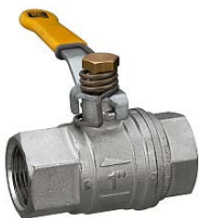
03-117 93AS Muffen-Kugelhahn Federrückstellung/ ball valve both ends female thread spring return fail-safe
